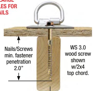
Nails/Screws min. fastener penetration 2.0"
