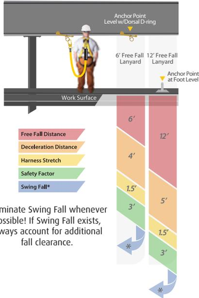
**Swing Falls:** Prior to installation or use, make considerations for eliminating or minimizing all swing fall hazards. Swing falls occur when the anchor is not directly above the location where a fall occurs. Always work as close to in line with the anchor point as possible. Swing falls significantly increase the likelihood of serious injury or death in the event of a fall.
