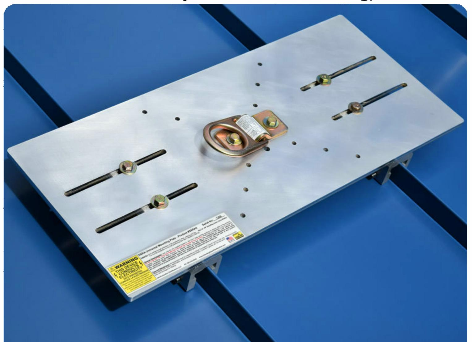
The SSRA3 Anchor Plate is a universal mounting plate constructed of 6061-T6 aluminum and professionally tested to over 10,000 lbs. It can be used to mount anything to a standing seam roof, including fall protection equipment. It is pre-drilled with 4 holes to accept the Falltech 7414 D-Ring (included) mounted either vertically for standard anchoring or mounted horizontally for Horizontal Lifeline attachment.
