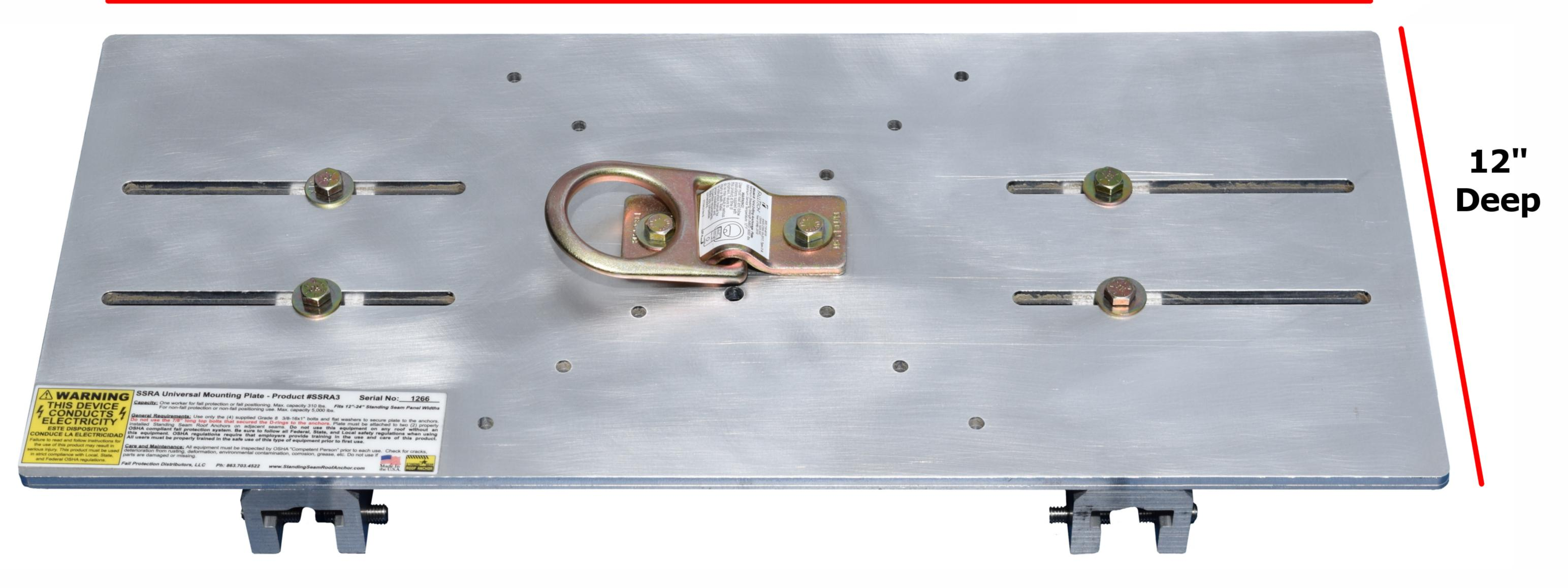
Overall plate dimension are 12"x27" with a 11"x12" mounting area between the slide grooves. The SSRA3 Anchor Plate will fit all compatible standing seams 12" - 24" wide.
